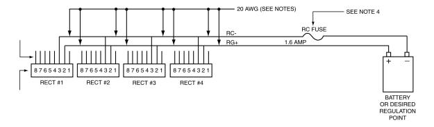
Figure 7 · No controller, remote sensing connection for 8-pin signal cable shelves
